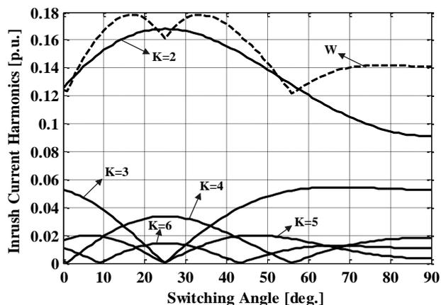
Fig. 4. Changes of harmonic currents and W index with respect to the switching angle.
