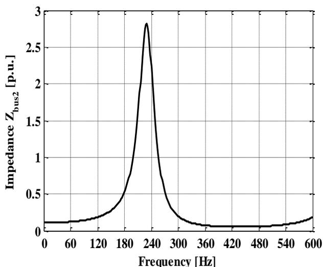
Fig. 3. Impedance at bus 2.
