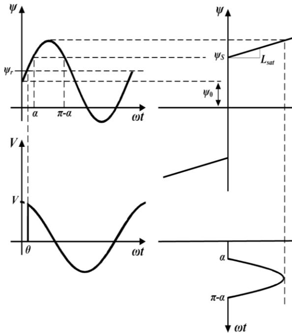
Fig. 1. Simplified transformer magnetization characteristic.
