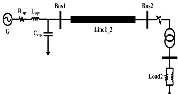
Fig. 2. Sample system for transformer energization study. G: generator,  $R_{eqv}$ : equivalent resistance,  $L_{eqv}$ : equivalent inductance, and  $C_{eqv}$ : equivalent capacitance.
