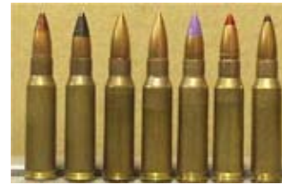
Fig. 2 7.62 mm match ammunition with a diameter of 0.30 caliber representative small bullet types.
