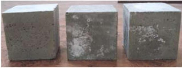
Figure 2. Geopolymer mortar specimens after 3 weeks exposure.
