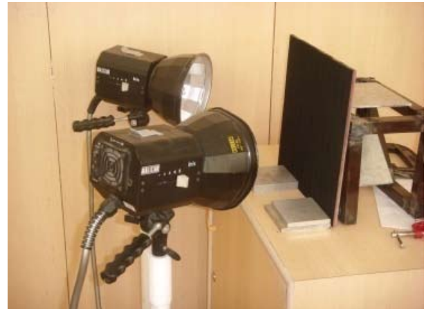
Figure 4. Infrared Thermography setup for the measurement of delamination occurred during milling.
